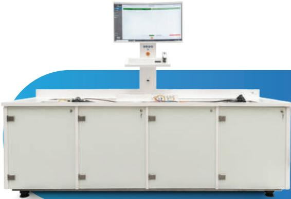
Semi automatically pre cleans multiple endoscopes at the same time with 100% traceability and this avoids the formation of biofilm
